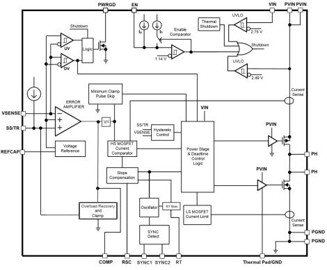
Fig. 2 TPS7H4001-SP functional block diagram.
