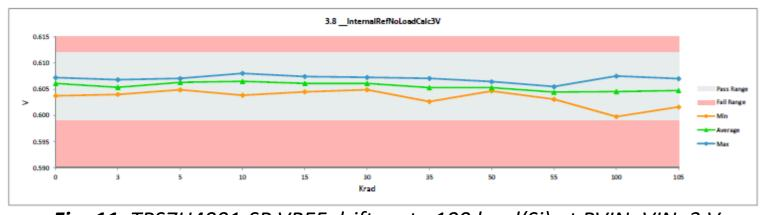
Fig. 11. TPS7H4001-SP VREF drift up to 100 krad(Si) at PVIN=VIN=3 V.
