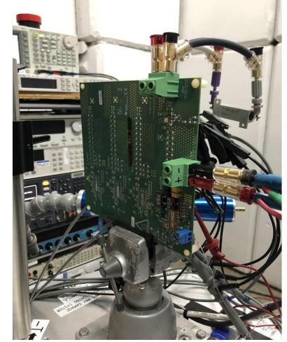
Fig. 3. Photograph of the TPS7H4001-SP Fig. 4. Block diagram of the setup used for the mounted on the TPS7H4001EVM-CVAL in front SEE testing at the TAMU cyclotron facilities. of the heavy-ion beam port exit at the TAMU cyclotron facility.
