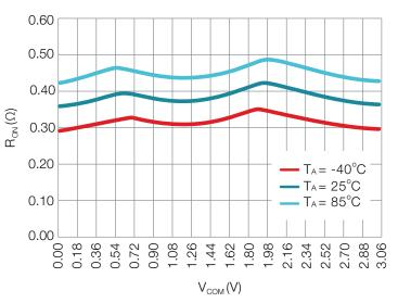
For IoT applications that are very sensitive to  $R_{oN}$  shifts, select switches where the  $R_{oN}$  does not change drastically over the operating voltage range expected for that application. Do consider lower  $R_{oN}$  switches with relatively flat  $R_{oN}$  over voltage and temperature when selecting devices for IoT.
