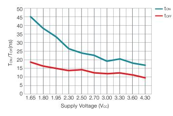
Figure 8. Example of Ton and TOFF curves from a quad-SPDT switch.
