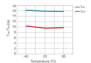
$T_{ON}$  and  $T_{OFF}$  vs Temperature (V<sub>CC</sub> = 4.3 V)
