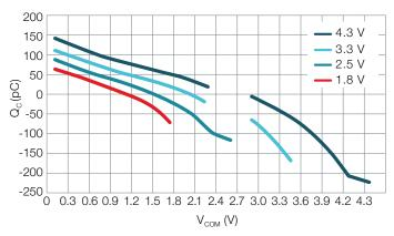
*Figure 6.* Example of charge injection specification from a quad-SPDT switch.
