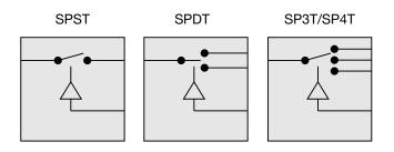
Figure 4. Examples of three common signal switch configurations.
