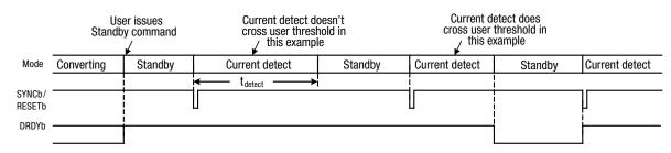
Figure 4. ADS131M04 current detection mode examples.
