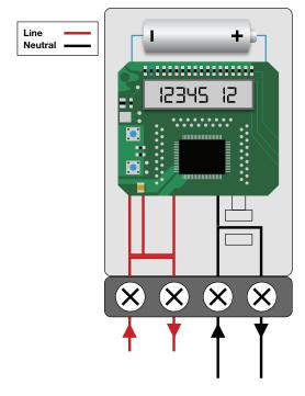
*Figure 1. Example electricity meter configuration under normal operation.*
