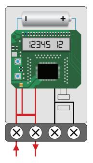
*Figure 2. Example electricity meter configuration with neutral disconnected.*
