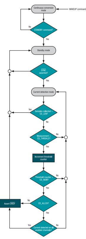
*Figure 3.* The current detection mode flow chart of the ADS131M04.
