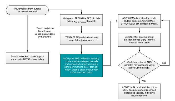
Figure 5. Sequence of events after power failure.
