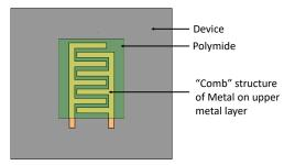
Figure 1-2. Capacitive Humidity Sensing Element
