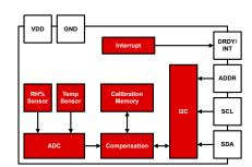
Figure 1-3. Internal Block Diagram of HDC2
