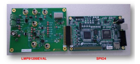
Figure 2 Sensor AFE evaluation platform
