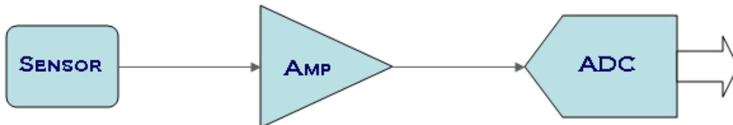
Figure 1-1: ADC Channel.
