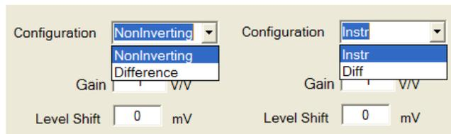
Figure 3-10: Amplifier Selection and Level Shift Value.
