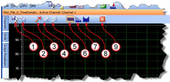
Figure 6: WaveVision 5 plot window controls
