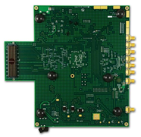
Figure 19: Bottom of ADC08D1520RB showing FMC port
