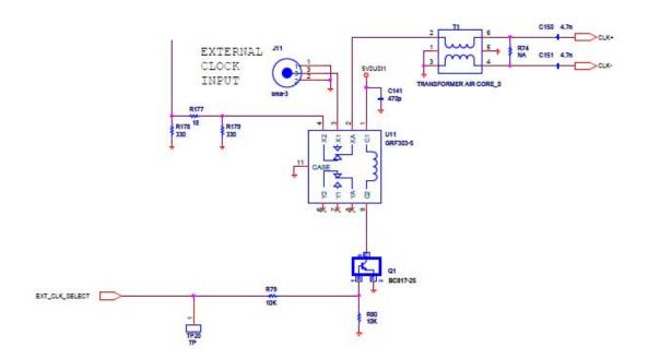
Figure 15. External / internal clock selection circuit on ADC08D1520RB
