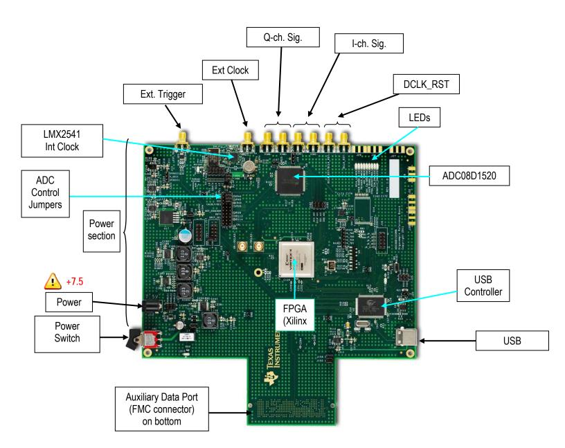
Figure 1: ADC08D1520RB Board Layout
