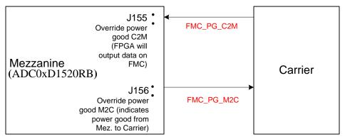
Figure 18: Explanation of Power Good override jumpers for FMC port
