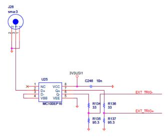
Figure 17: Trigger circuit on reference board
