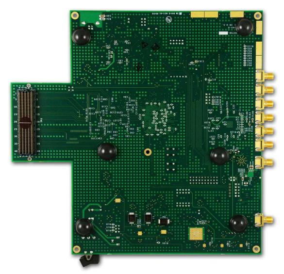
Figure 19: Bottom of ADC0XD1520RB showing FMC port
