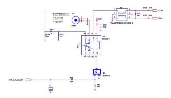
Figure 15. External / internal clock selection circuit on ADC0XD1520RB
