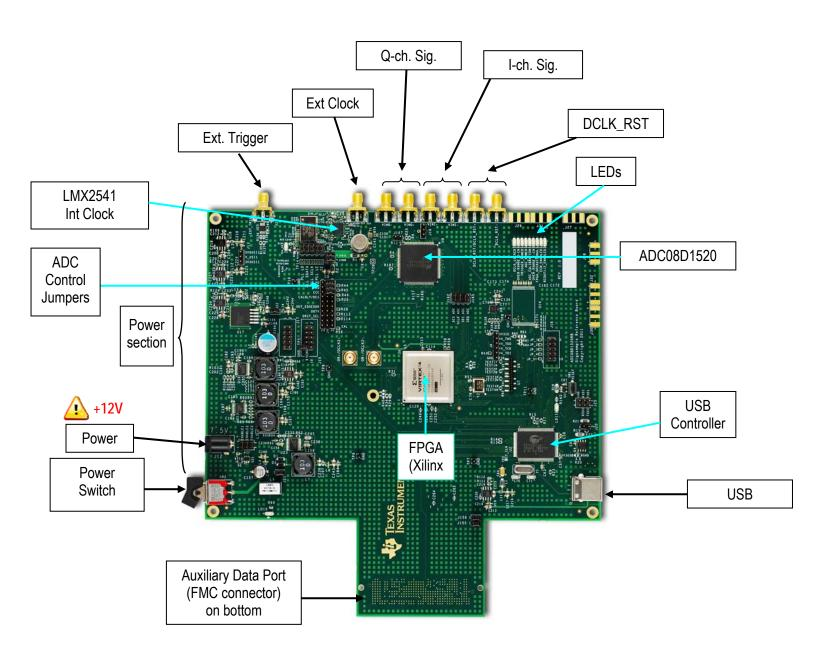
Figure 1: ADC0XD1520RB Board Layout
