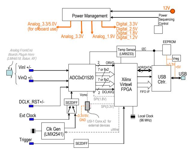
Figure 16: ADC0XD1520RB System Block Diagram
