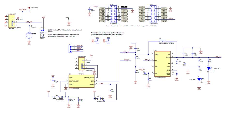
Pull down resitance (RD) on DONE pin Whe the EVM is used stand alone, J2.1 and J2.2 are shorted When the EVM is used with the launchpad (or other uC) J2.1 and J2.2 are NOT shorted
