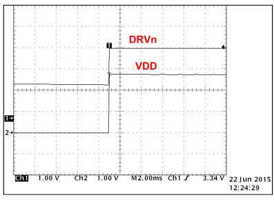
Figure 5. Boost Converter Input (DRVn) and Output (VDD)
