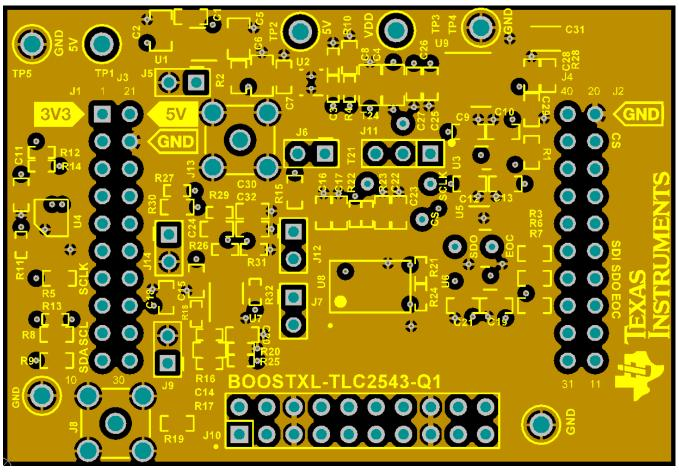
Figure 15. BOOSTXL-TLC2543 Ground Layer
