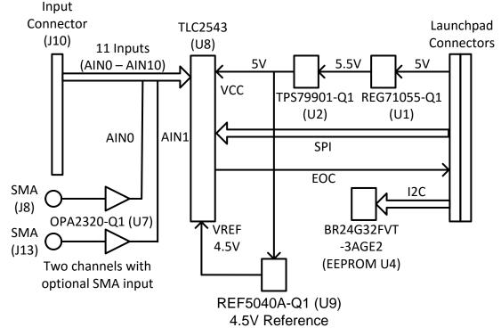
Figure 1. BOOSTXL-TLC2543 EVM Block Diagram
