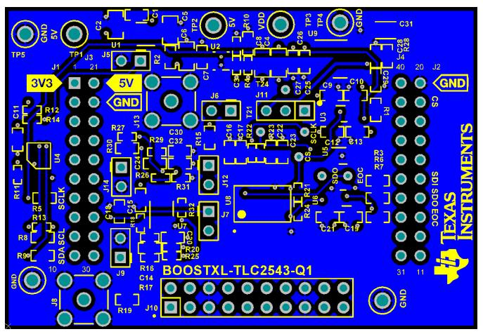
Figure 17. BOOSTXL-TLC2543 Bottom Layer Routing
