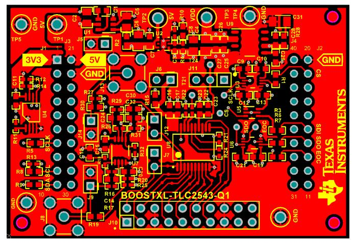
Figure 14. BOOSTXL-TLC2543 Top Layer Routing
