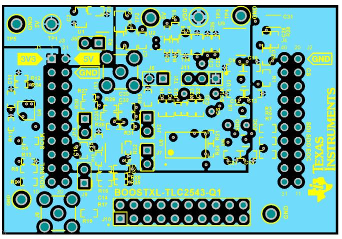
Figure 16. BOOSTXL-TLC2543 Power Layer
