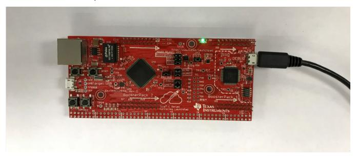
Figure 6. TM4C1294 LaunchPad<sup>™</sup> Development Kit Software Programming Setup
