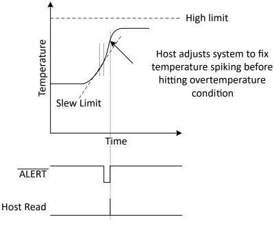
Figure 2-1. Slew Rate Warning
