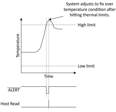
Figure 1-1. Traditional Threshold Alert
