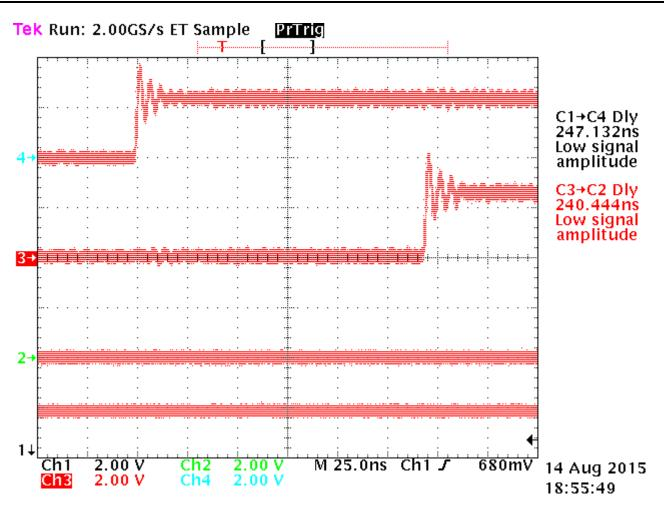
Figure 5. Start of Frame Measurement (Zoom)
