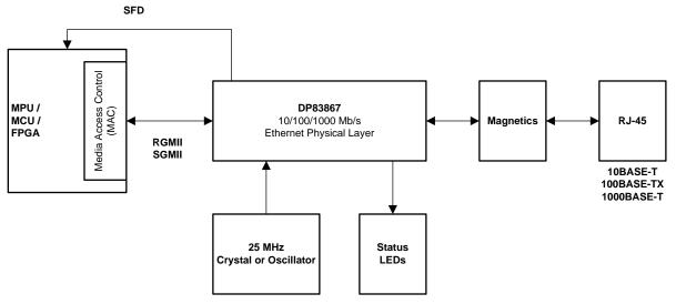
Figure 2. DP83867 SFD Connection Diagram
