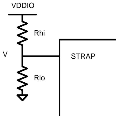
**Figure 1. DP83867 Strapping Configuration**
