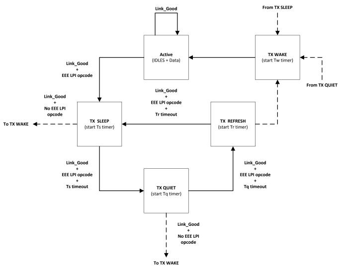
Figure 3. Transmit Path LPI State Diagram
