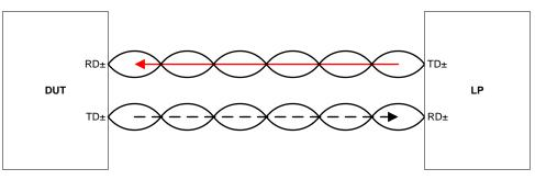
Figure 6. LP Active and DUT in LPI
