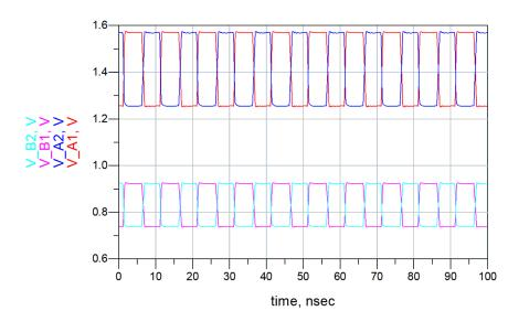
Figure 3-3. Simulation Results for Devices Without Internal Termination
