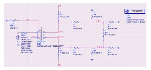
Figure 4-2. Schematic for Receivers With Internal Termination
