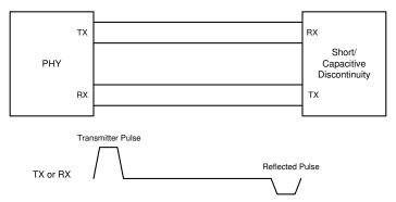
Figure 1-2. Short Circuit Cable
