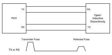
Figure 1-1. Open Circuit Cable
