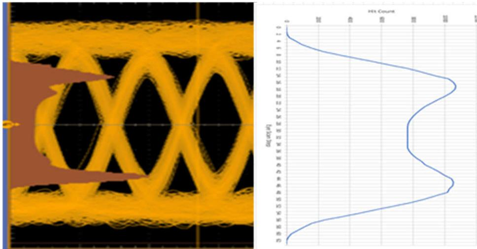
**Figure 3-5. Histogram Plot of Captured Eye After Redriver vs. Eye Scan Capture Plot**
