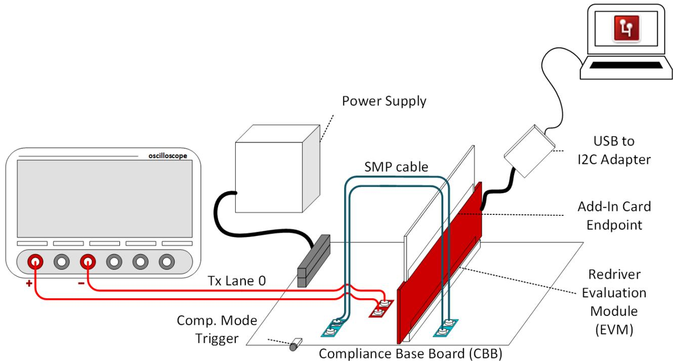
**Figure 4-1. PCIe TX Compliance Setup**
