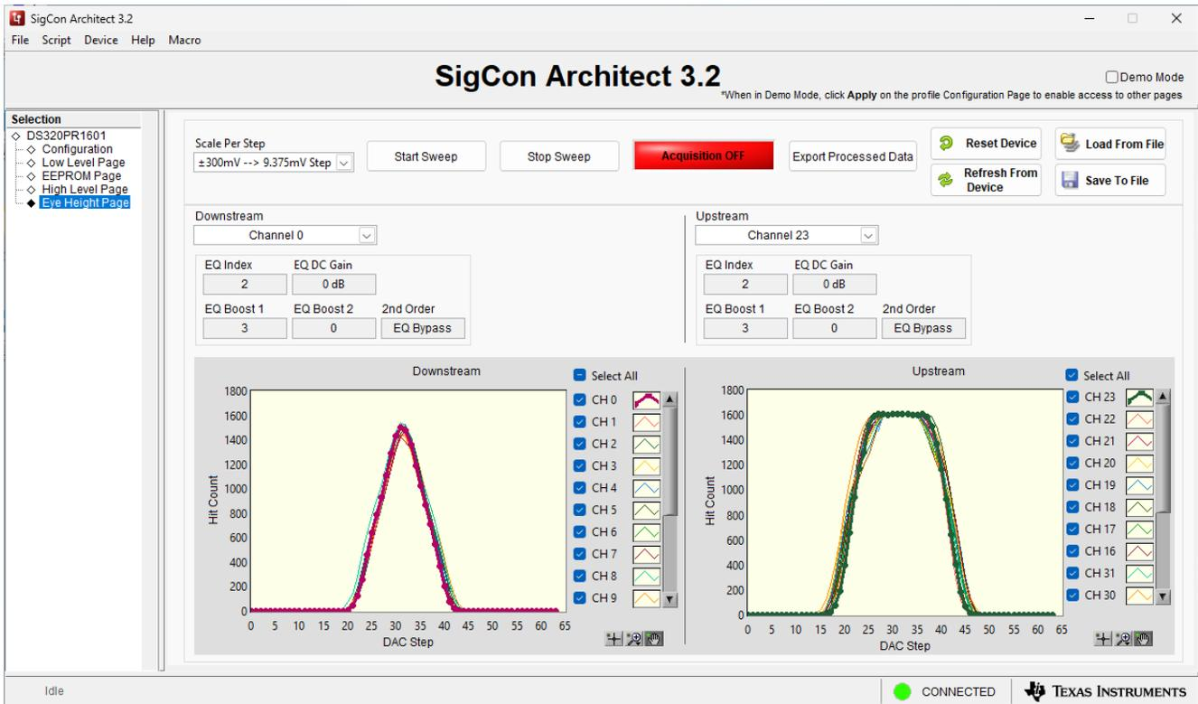
**Figure 5-3. Example Eye Scan Plot Capture Using SigCon Architect**
