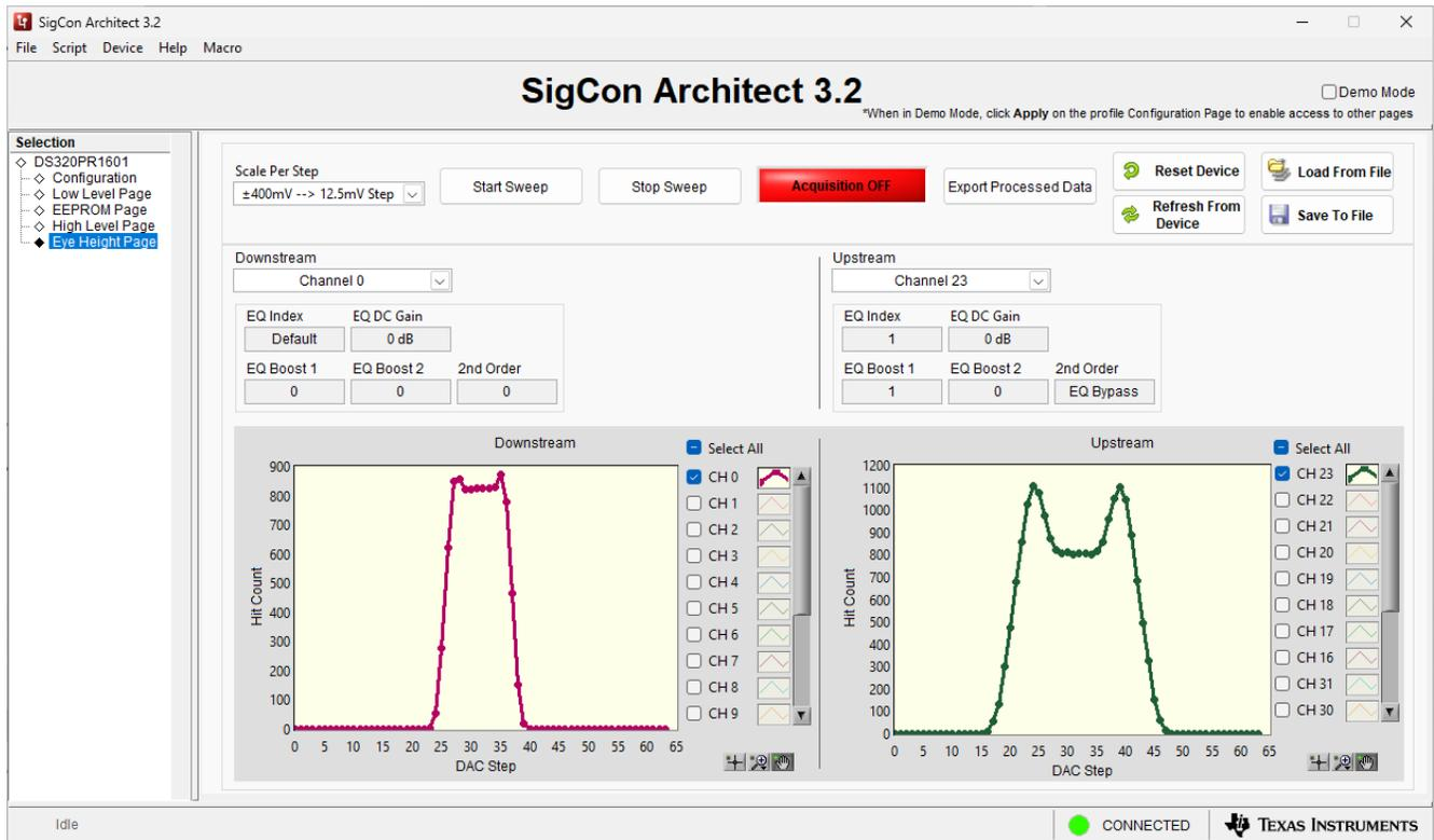
Figure 4-5. Example System Eye Scan Plot in the SigCon Architect GUI
