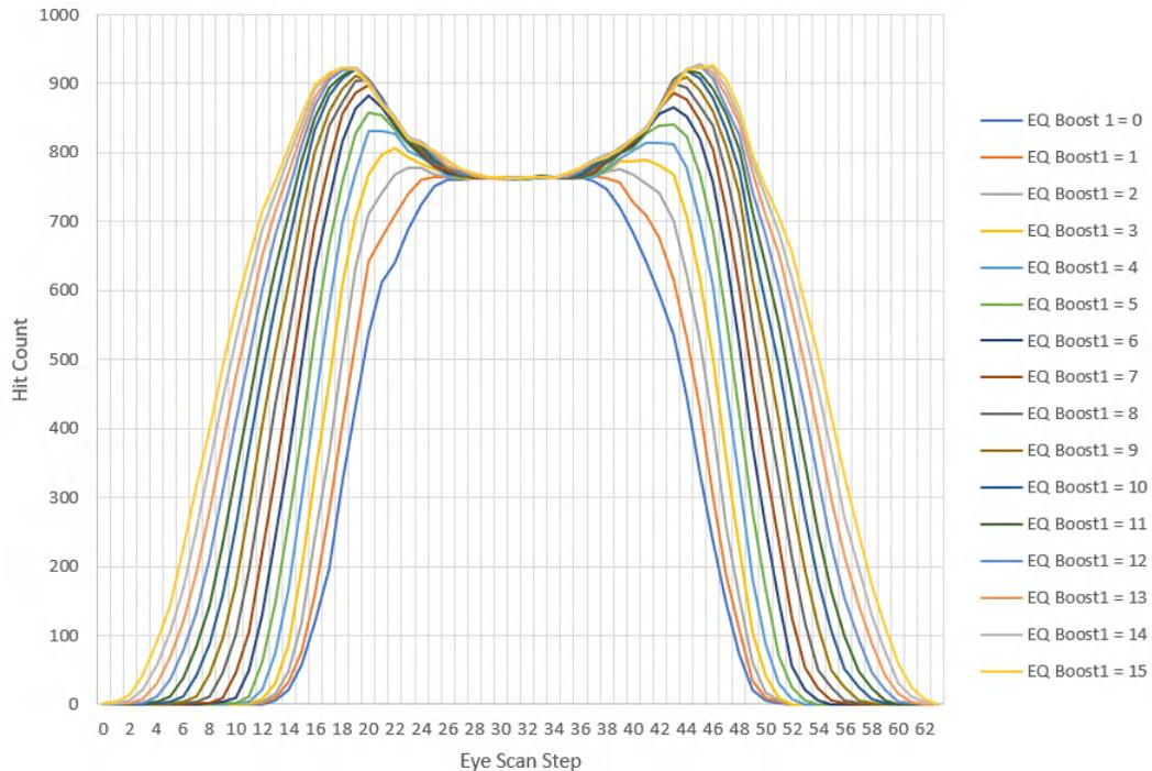
**Figure 3-6. Eye Scan Results of Varying EQ Boost 1 Settings**
