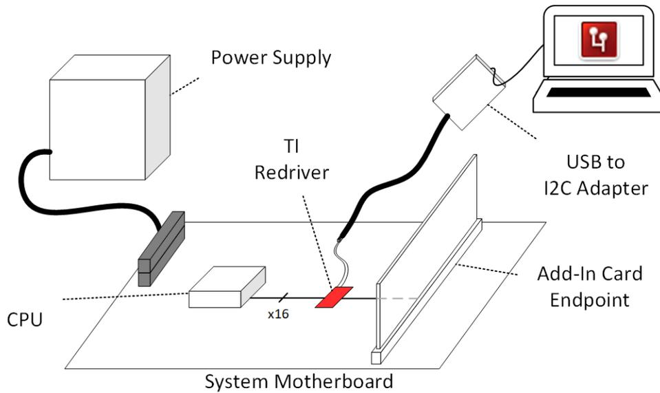
**Figure 4-4. PCIe System Configuration Using a TI PCIe Redriver on a Motherboard**
