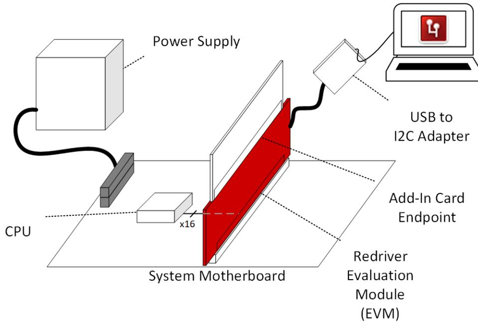
**Figure 4-3. PCIe System Configuration Using a TI PCIe Redriver EVM**
