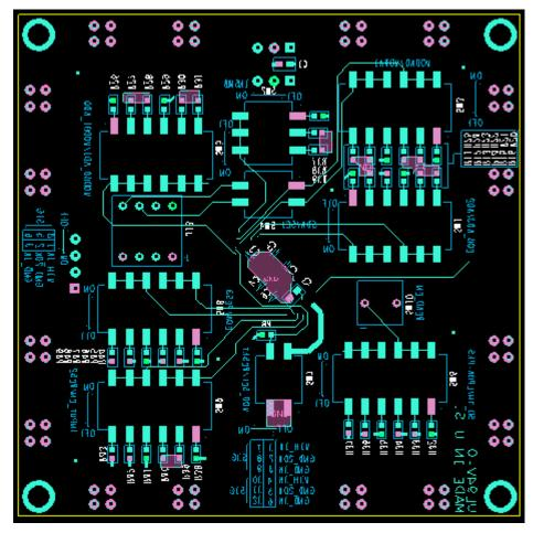
Figure 6-2. Bottom Assembly Layer
