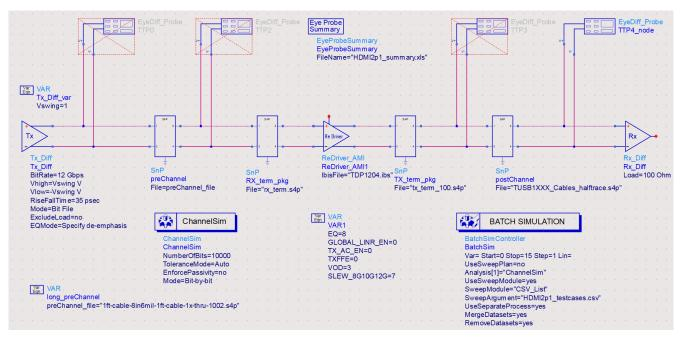
Figure 4-1. ADS Simulation Setup
