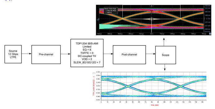
Figure 4-2. Simulation Results and Bench Correlation
