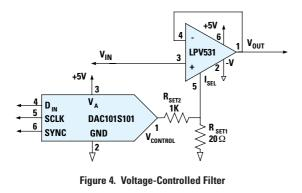
When the control voltage is near 0V, the  $I_{SEL}$  current is determined by the parallel combination of the two resistors  $R_{SET1}$  and  $R_{SET2}$ . When the control voltage is greater then zero, the Thevenin Equivalent voltage and resistance at the  $I_{SEL}$  pin will determine the  $I_{SEL}$  current. The following equation can be used to calculate the amplifier's supply current:
