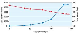
Figure 1. LPV531 Gain Bandwidth vs Supply Current
