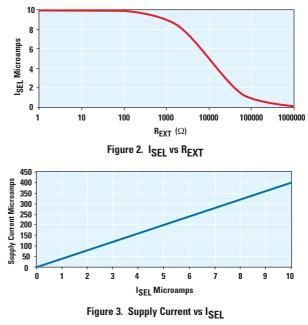
To implement a voltage controlled filter, the  $I_{SEL}$  current must be made dependent on voltage rather then a resistor.
