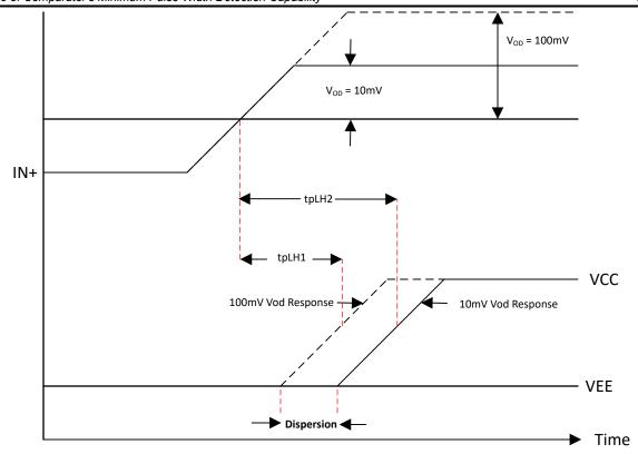
Figure 3-2. Input Overdrive Dispersion Plot
