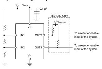
Figure 9. Multi-Level Voltage Detection using TLV4062 and TLV4082
