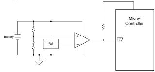
Figure 6. Undervoltage Detection using a Comparator + External Reference
