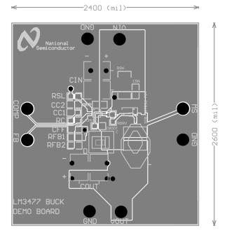
Figure 5-1. LM3477 Evaluation Board PCB Layout (Top Side)
