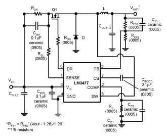
Figure 1-1. LM3477 Buck Converter
