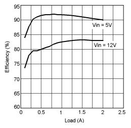
Figure 2-1. Efficiency vs Load V<sub>OUT</sub> = 3.3 V
