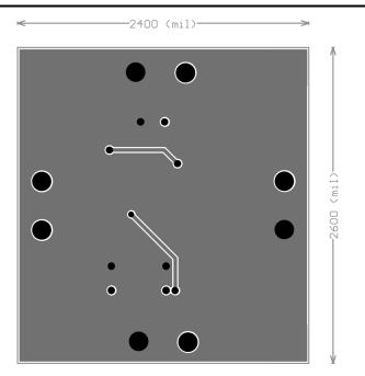
Figure 5-2. LM3477 Evaluation Board PCB Layout (Bottom Side)
