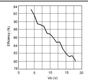
Figure 2-2. Efficiency vs V<sub>IN</sub> V<sub>OUT</sub> = 3.3 V, I<sub>OUT</sub> = 2 A
