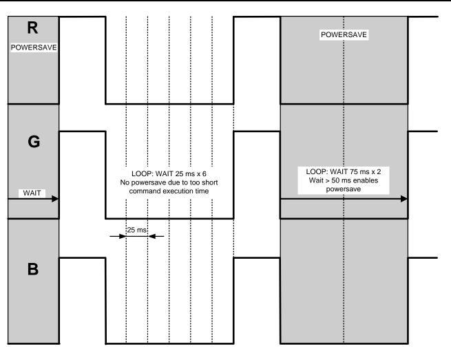
Figure 5. Power Save Sequence With Long and Short Wait Commands
