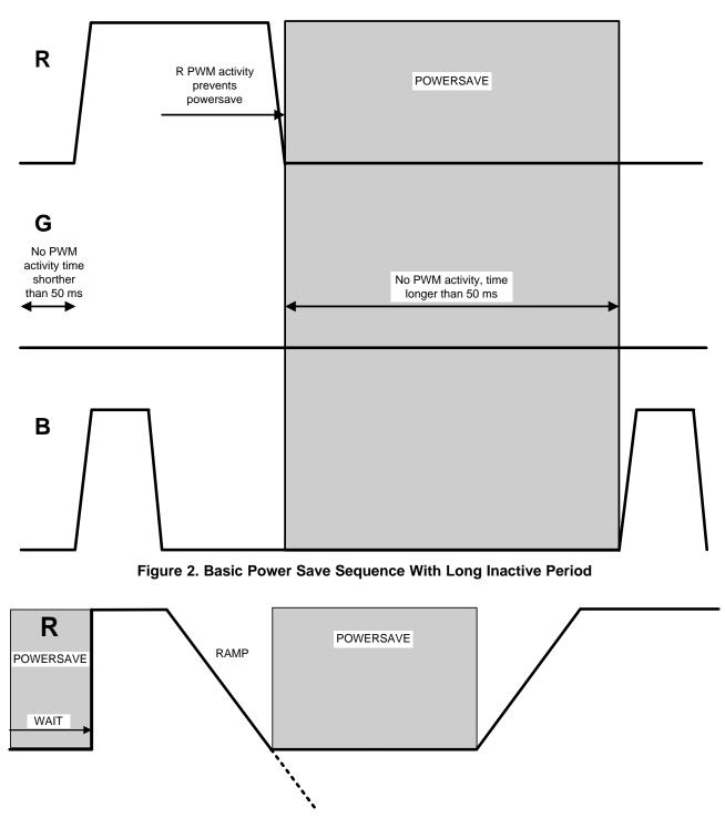
Figure 3. Power Save Sequence With a Ramp Command Used as Combined Ramp/Wait
