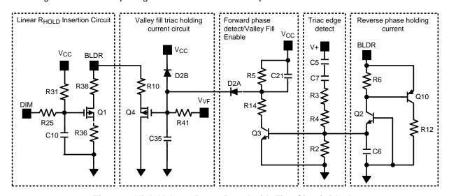
Figure 9. High Voltage Demo Board with Five Circuit Blocks
