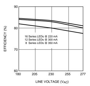
Figure 2. Efficiency Plot
