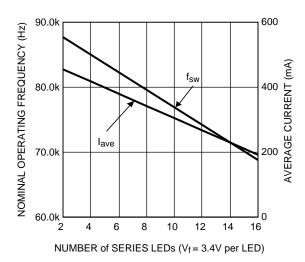
Figure 10. Output Variation w/0 Component Adjustment
