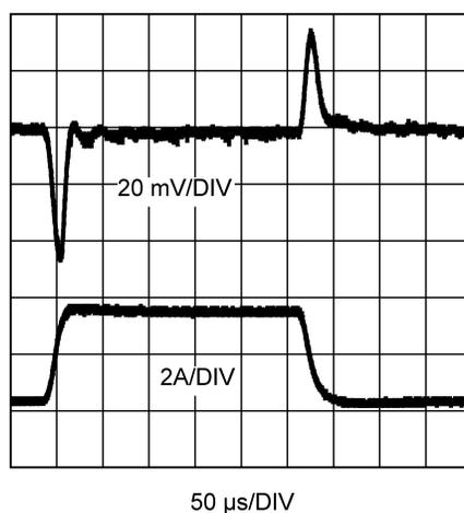
**Figure 16. Load Transient Response**
