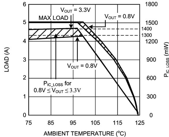
Figure 7. Current Derating vs. Ambient Temperature
