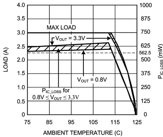
**Figure 5. Current Derating vs. Ambient Temperature**
