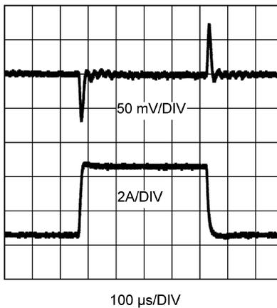
**Figure 18. Load Transient Response**
