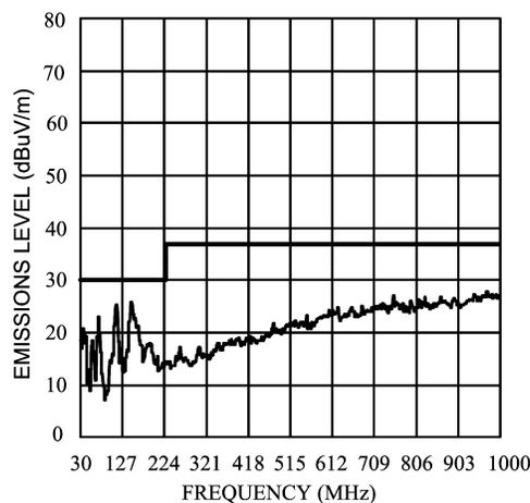
**Figure 21. Radiated Emissions (EN55022, Class B)**
