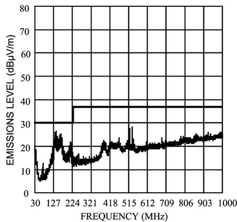
**Figure 20. Radiated Emissions (EN55022, Class B)**
