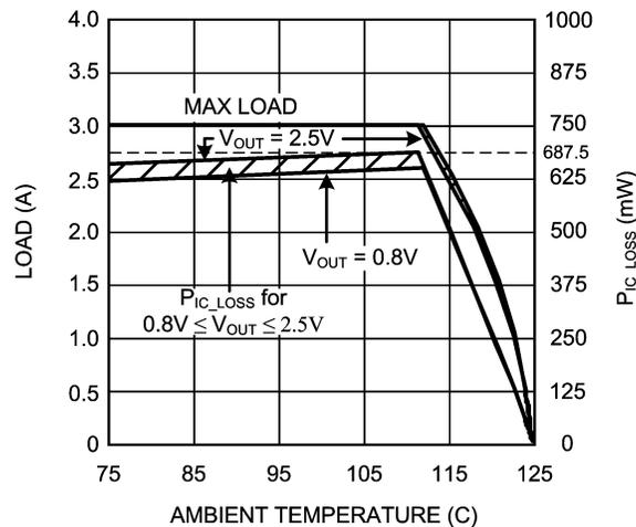
Figure 8. Current Derating vs. Ambient Temperature
