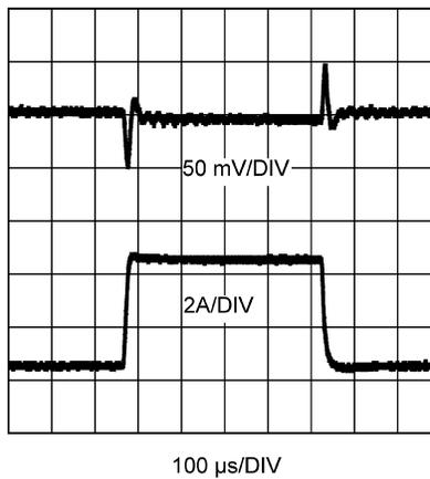
**Figure 17. Load Transient Response**
