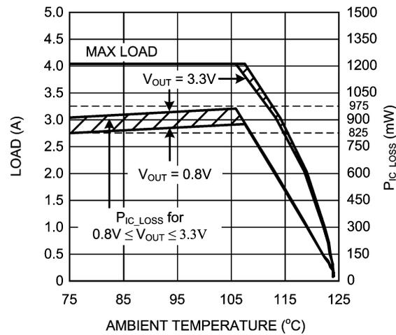
Figure 6. Current Derating vs. Ambient Temperature
