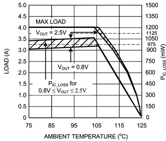
Figure 9. Current Derating vs. Ambient Temperature
