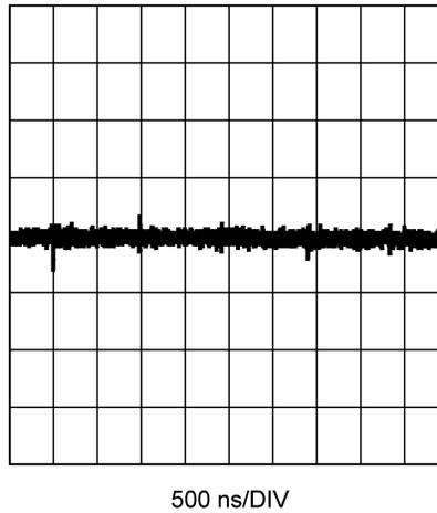
**Figure 14. Output Voltage Ripple**
