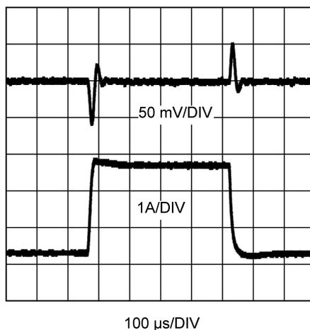
**Figure 15. Load Transient Response**
