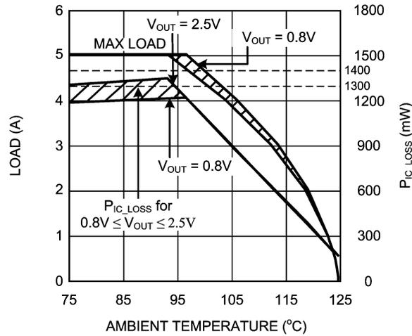
Figure 10. Current Derating vs. Ambient Temperature
