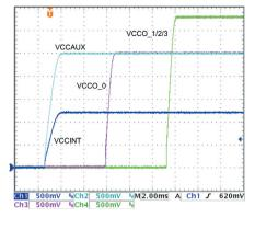
Figure 3. FPGA Solution - Startup
