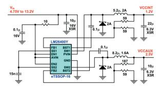
Figure 2. FPGA Power - VCCINT and VCCAUX
