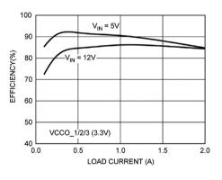
Figure 4. FPGA Solution - Efficiency
