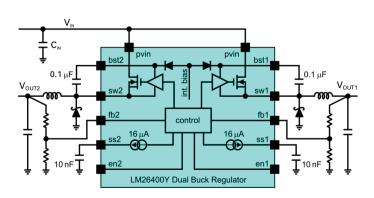
Figure 1. Simplified View of the LM26400Y Regulator
