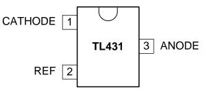
Figure 1. 3-Pin SOT-23 Package (Top View)
