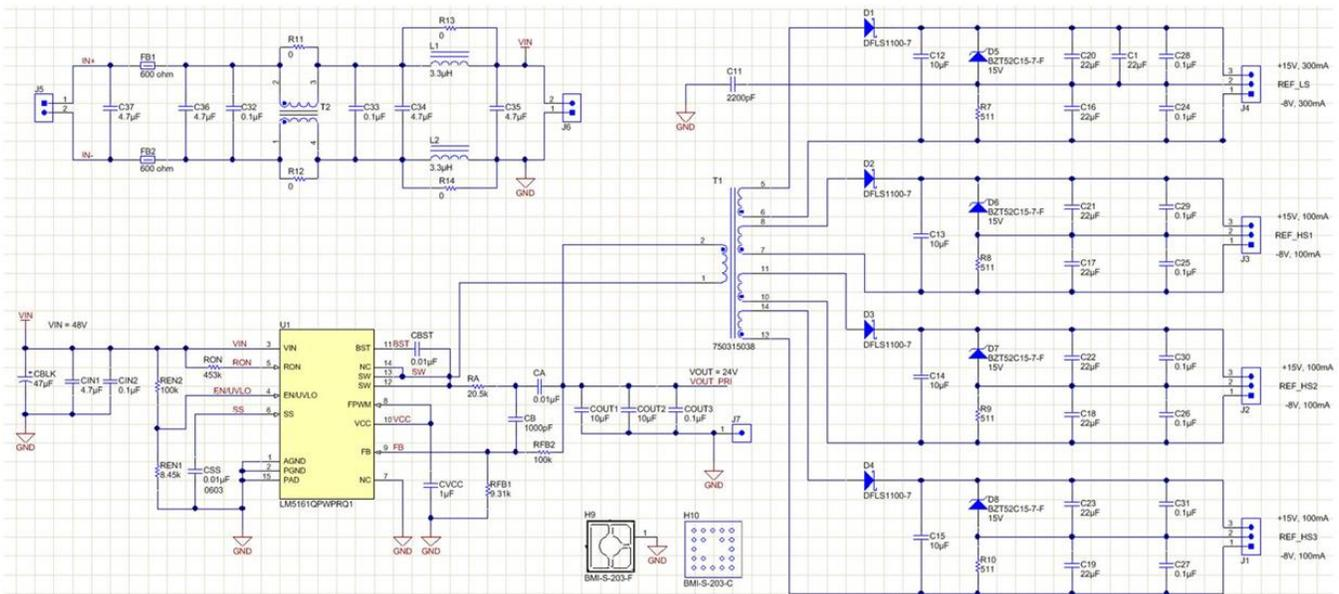
Figure 5. 48-V Flyback IGBT Supply Design: Schematic
