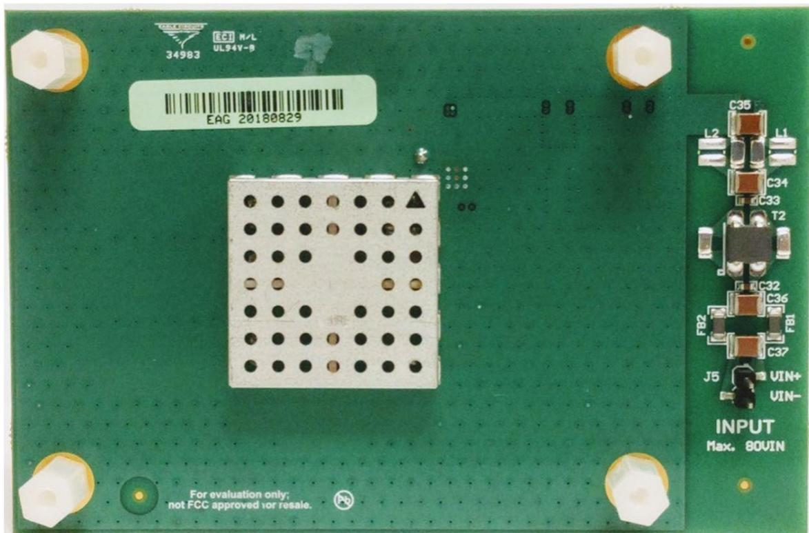
Figure 11. 48-V Flyback IGBT Supply Design: Board - Bottom
