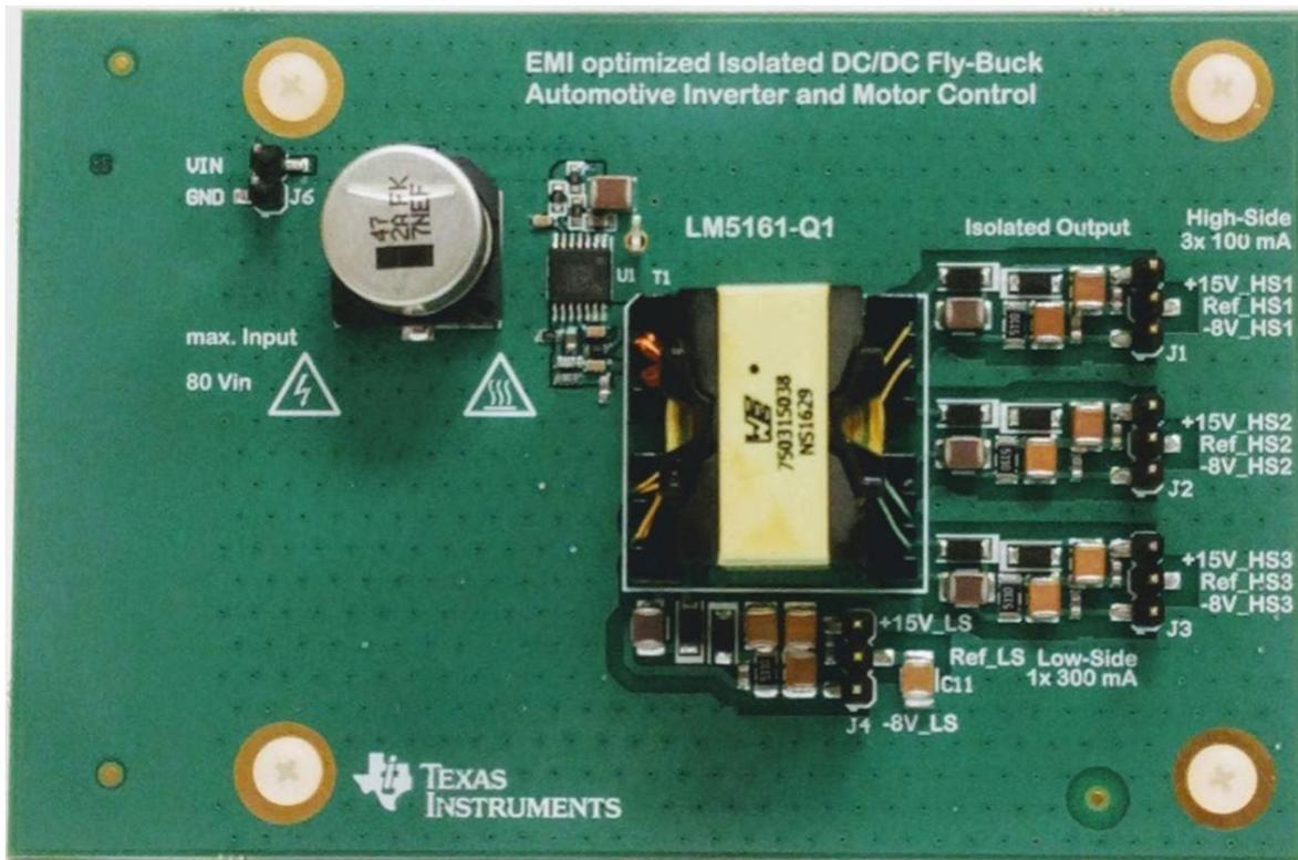
Figure 10. 48-V Flyback IGBT Supply Design: Board - Top
