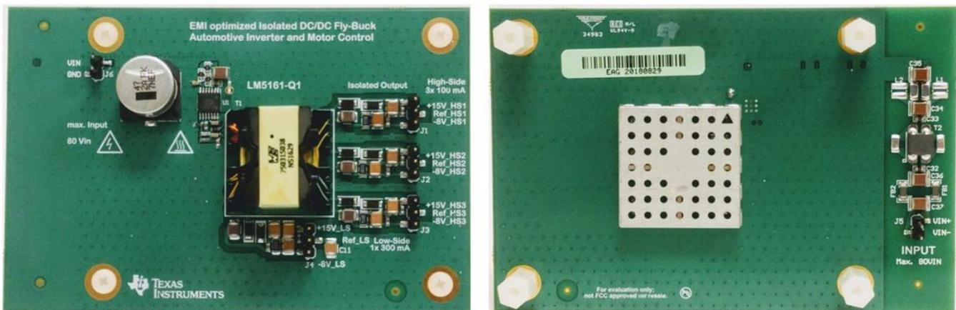
Figure 2. 48-V Flybuck IGBT Supply Design: Board Front (left) and Back (right)
