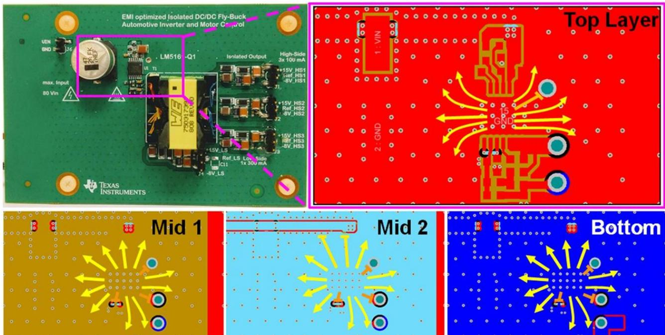
Figure 25. 48-V Optimized Board Layout Showing Heat Path
