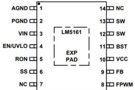
Figure 4. Pinout Comparison: LM5160 (left) vs LM5161 (right)
