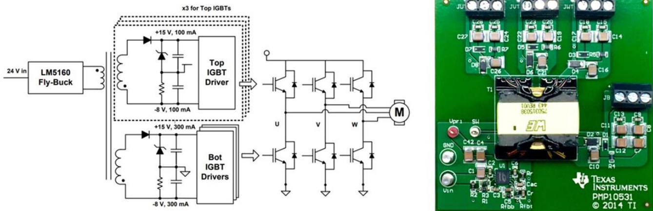
**Figure 3. [TIDA-00199](#) 24-V Flyback IGBT Supply Design: Simplified Schematic (left) and Board (right)**
