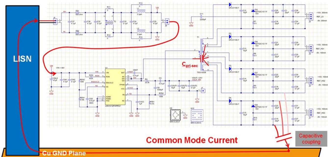
Figure 18. Common-Mode Current in EMI Test – Equivalent Schematic
