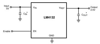
Figure 4-2. Typical LM4132-Q1 Schematic
