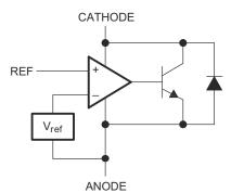
Figure 1-1. Equivalent Schematic
