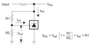
Figure 4-1. Test Circuit for V<sub>KA</sub> > V<sub>ref</sub>
