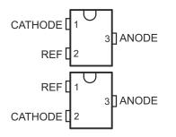
Figure 4-2. Pin Diagram for DBZ Package
