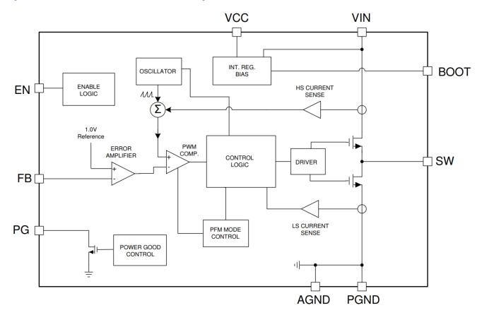
Figure 1-1. Functional Block Diagram: LM60430, LM60440
