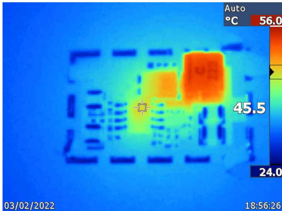
Figure 2-6. Thermal Rise on Experimental LM5013 PCB (110cm<sup>2</sup> , 4-Layer Board)
