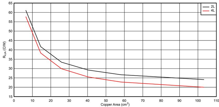
Figure 2-3. LM5013 R<sub>θJA</sub> vs. Copper Area
