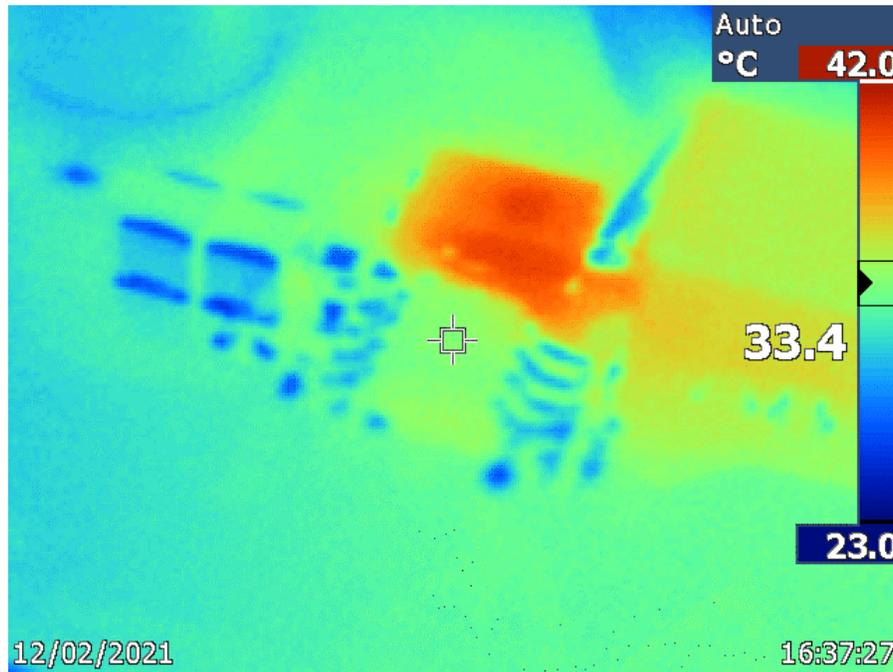
Figure 3-2. Diode Self-Heating Impact on Neighboring Regulator
