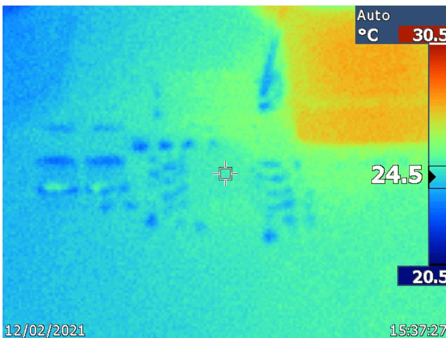
**Figure 3-1. Inductor Self-Heating Impact on Neighboring Regulator**
