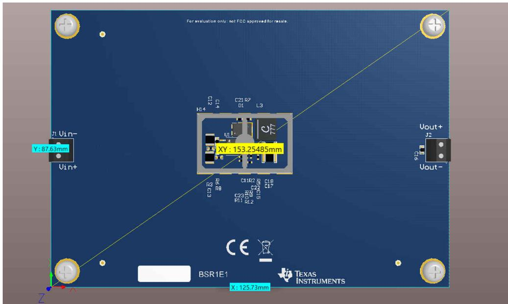
Figure 2-5. Experimental LM5013 PCB 3-D image
