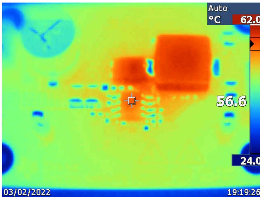
Figure 2-4. Thermal Rise on LM5013-Q1EVM (21.6cm<sup>2</sup>, 4-layer board)
