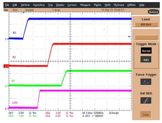
Figure 2-4. TPS650330-Q1 Programmable Power Up Sequence
