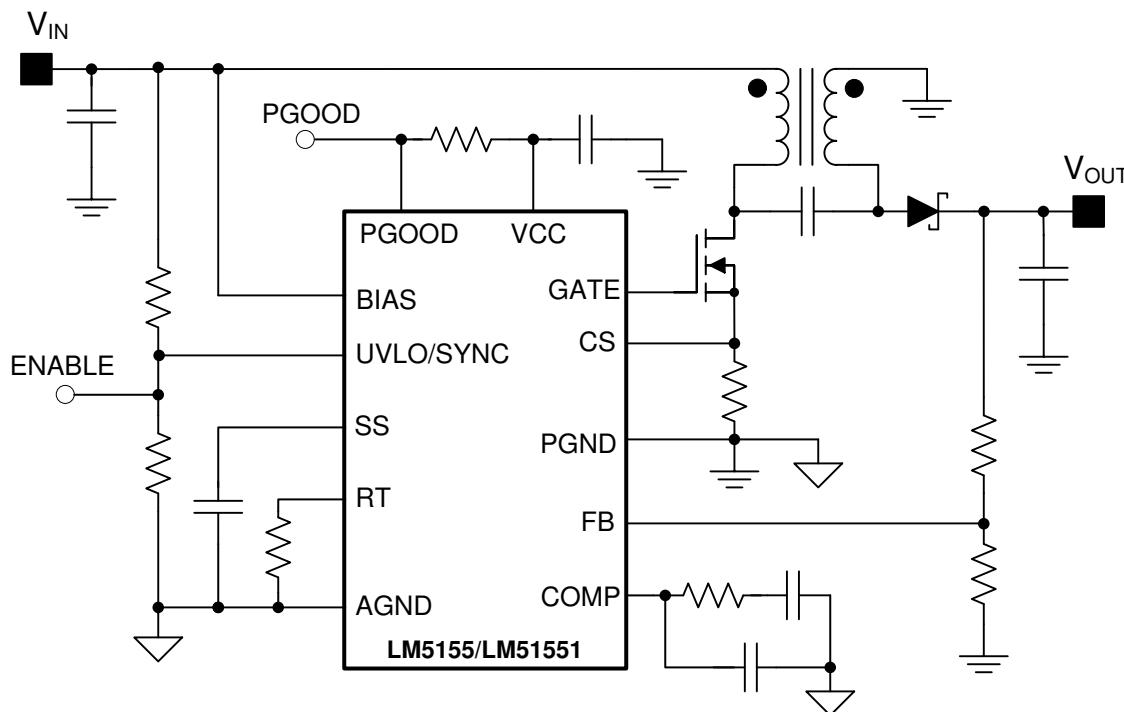
**Figure 4-1. Application Circuit**
