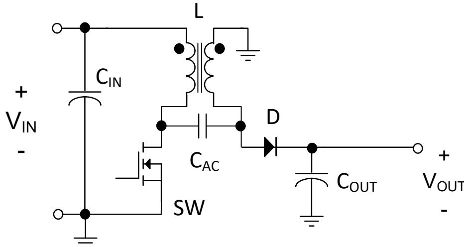
**Figure 1-1. Coupled Inductor SEPIC Power Stage**
