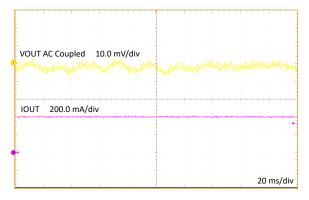
Figure 4-10. Output Voltage Ripple,  $V_{IN} = 24 V$ ,  $V_{OUT} = -12 V$ ,  $I_{OUT} = 410 mA$
