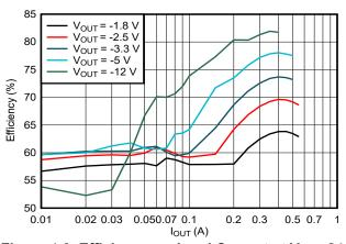
Figure 4-3. Efficiency vs. Load Current at V<sub>IN</sub> = 24 ν
