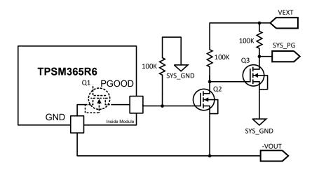
Figure 5-4. PGOOD Pin Level Shifter
