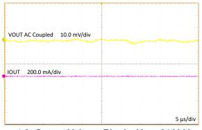
Figure 4-9. Output Voltage Ripple,  $V_{IN}$  = 24 V,  $V_{OUT}$ = -12 V,  $I_{OUT}$  = 0 mA
