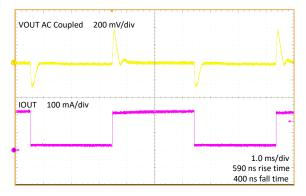
Figure 4-7. Load Transient Response, 100 mA to 410 mA With  $V_{IN}$  = 24 V,  $V_{OUT}$  = -12 V
