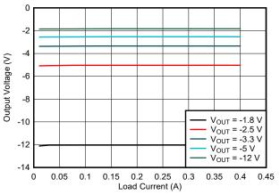
Figure 4-4. Load Regulation at V<sub>IN</sub> = 24 V
