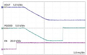
Figure 4-5. Start-up on  $V_{IN}$  = 24 V,  $V_{OUT}$  = -12 V, Expected Performance With no Level Shifters
