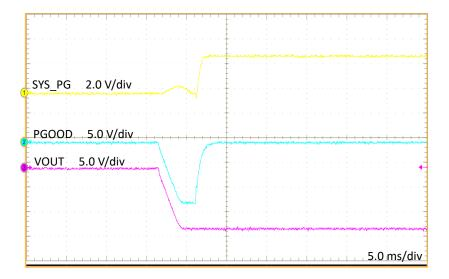
Figure 5-5. PG Pin Level Shifter on Start-Up
