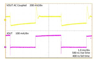
Figure 4-8. Load Transient Response, 0 mA to 410 mA With  $V_{IN}$  = 24 V,  $V_{OUT}$  = -12 V
