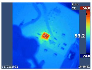
Figure 4-11. Temperature Response,  $V_{IN}$  = 24 V, V<sub>OUT</sub> = -5 V, I<sub>OUT</sub> = 450 mA
