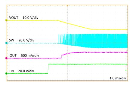
Figure 2-3. SW Node Voltage During Start-Up
