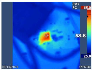
Figure 4-12. Temperature Response, V<sub>IN</sub> = 24 V,  $V_{OUT}$  = -12 V,  $I_{OUT}$  = 410 mA
