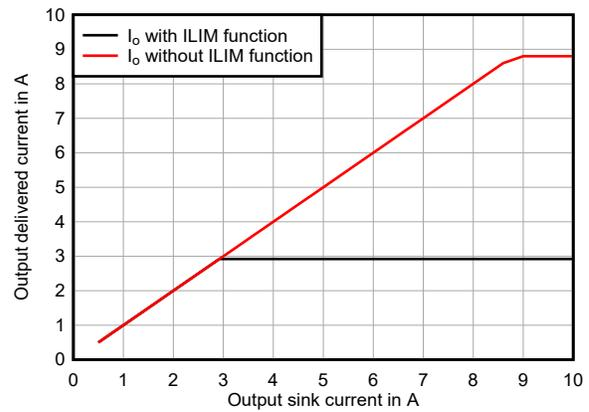
**Figure 7. ILIM Buck Mode  $V_{IN}$  24 V**
