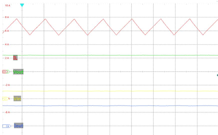
**Figure 4. Boost Mode Without ILIM Operation**
