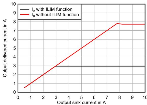
**Figure 8. ILIM Buck Boost Mode  $V_{IN}$  12 V**
