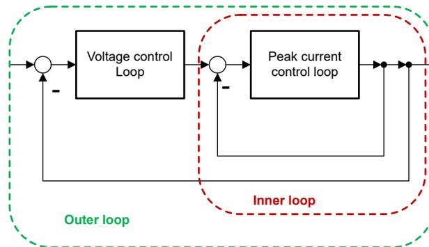
**Figure 1. Overview of Cascaded Control Loops**
