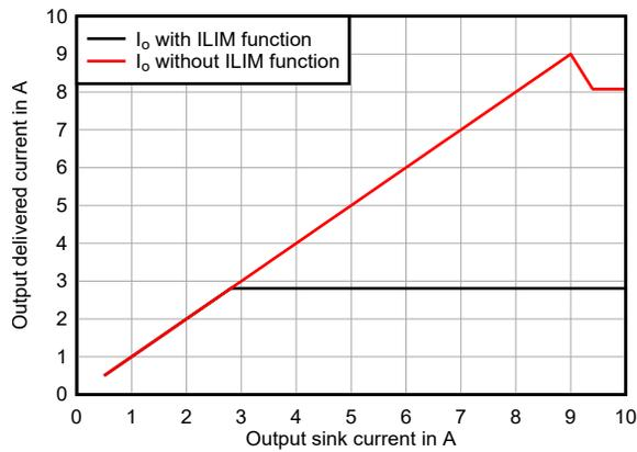
**Figure 6. ILIM Boost Mode  $V_{IN}$  6 V**
