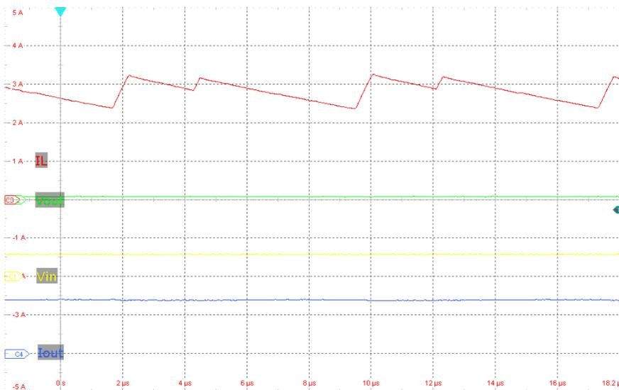
**Figure 5. Boost Mode with ILIM Operation**
