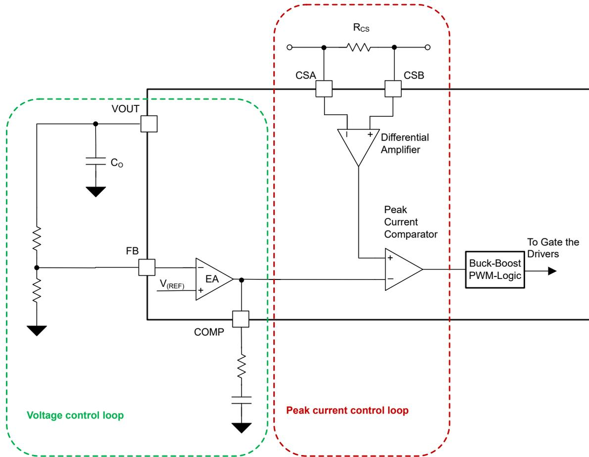
**Figure 2. Block Diagram for Inductor Peak Current Loop**
