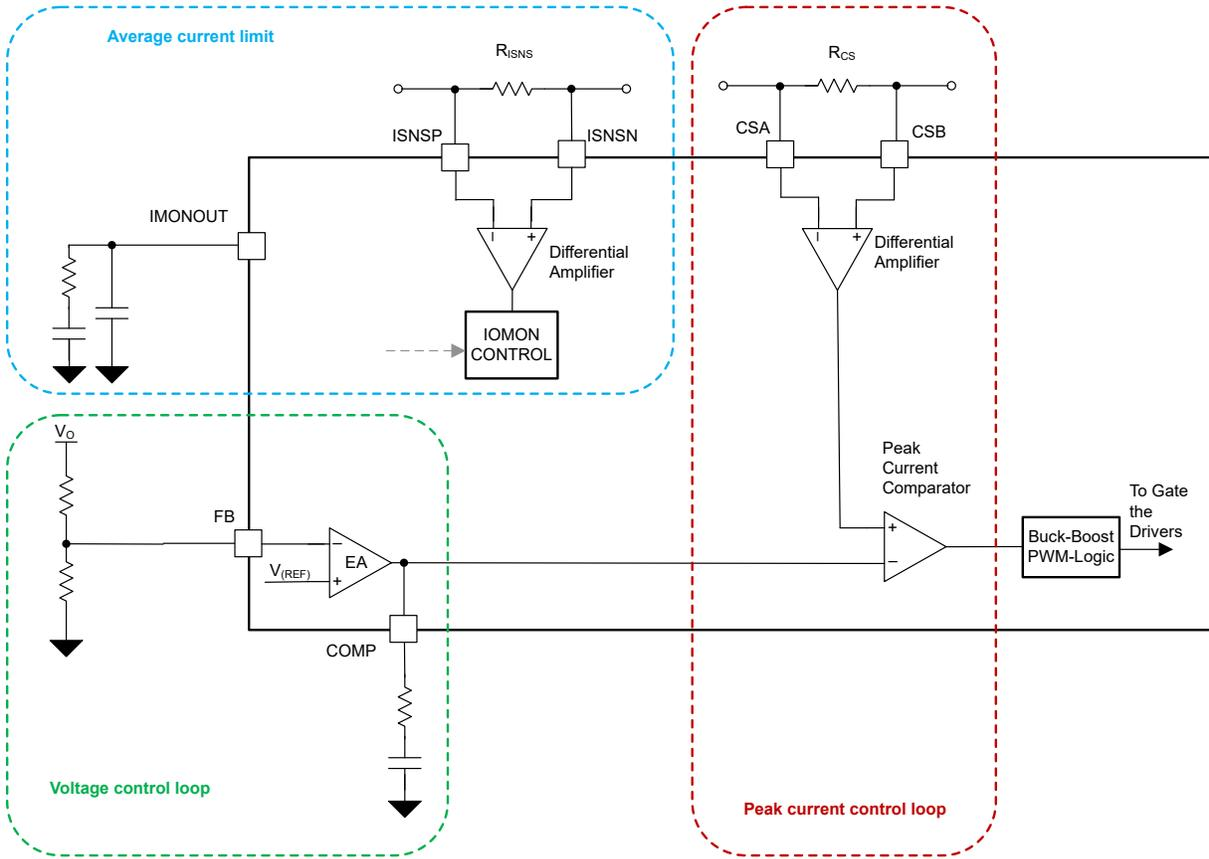
**Figure 3. Block Diagram for Average Current Limit Loop**
