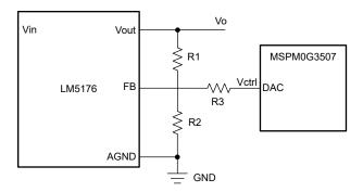
Figure 2-2. Control of Vout Using MCU
