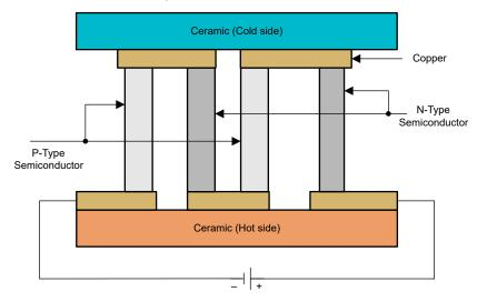
Figure 1-1. Structure of TEC Element
