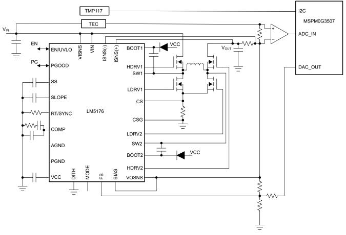
Figure 2-1. Block Diagram of TEC Design Using LM5176
