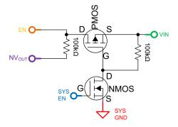
Figure 5-1. EN Pin Level Shifter
