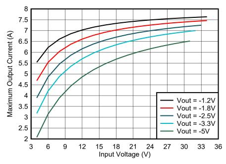
Figure 1-2. Recommended Maximum Output Current for TPSM63610
