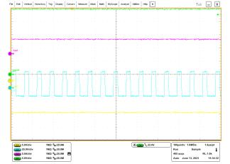
Figure 4-5. Load Transient With 2.5-A to 5-A Load Step at -12 Vout
