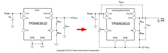
Figure 1-1. Converting From Buck to Inverting Buck Boost Topology
