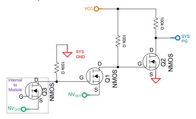
Figure 5-2. PGOOD Pin Level Shifter
