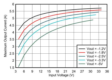
Figure 1-3. Recommended Maximum Output Current for TPSM63608
