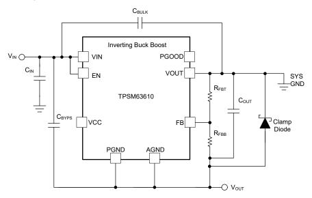
Figure 2-1. TPSM63610 Inverting Buck-Boost Schematic
