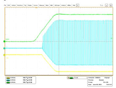
Figure 2-2. Typical SW Node Characteristics During Start-Up
