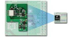
Discrete driver solution and integrated LM5113 driver. The LM5113 delivers tremendous efficiency and PCB area savings compared to discrete implementations.
