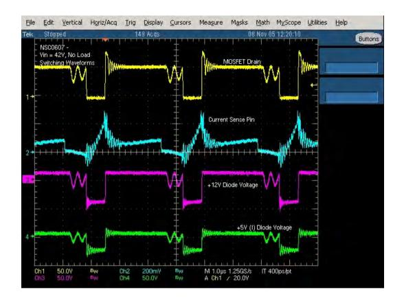
FIGURE 14. Switching waveforms, Vin=42V
