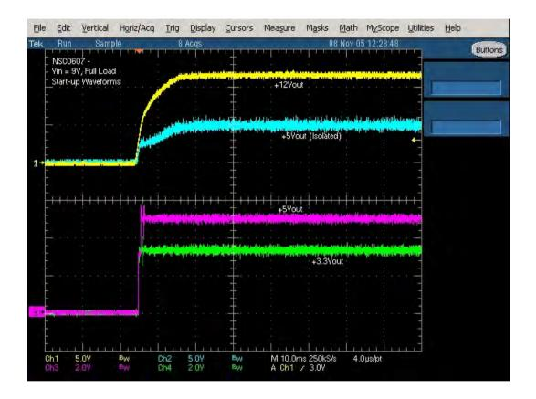
FIGURE 13. Start up waveforms, Vin=9V
