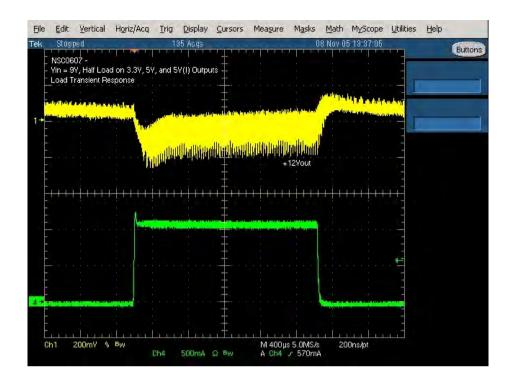
FIGURE 11. Load Transient, Vin=9V
