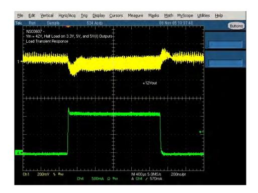
FIGURE 10. Load Transient, Vin=42V
