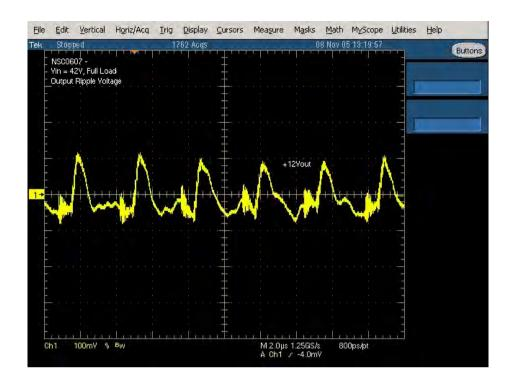
FIGURE 8. Output Ripple, Vin=42V
