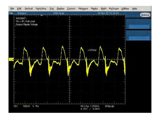
FIGURE 9. Output Ripple, Vin=9V
