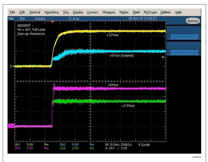
FIGURE 12. Start up waveforms, Vin=42V
