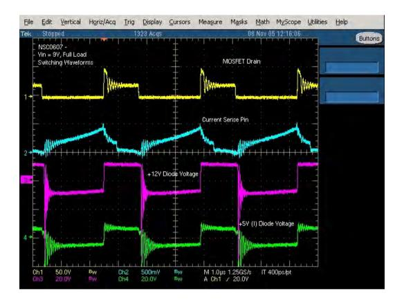
FIGURE 15. Switching waveforms, Vin=9V
