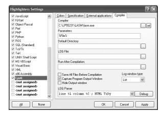
PSPad compiler settings for LP55231. Note: These variable names are all case-sensitive so, for example %File% will work, but %file% and %FILE% will fail to produce the expected results.
