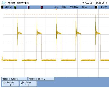
4. Test condition: The input voltage was set at 32V, and all four outputs were set at full load. Ch1 – Vd4 (+5V output diode voltage stress from cathode (-) to anode (+), 60V rating diode)
