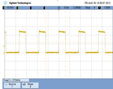
2. Test condition: The input voltage was set at 24V, and all four outputs were set at no load. Ch1 – Vsw (switch node voltage)
