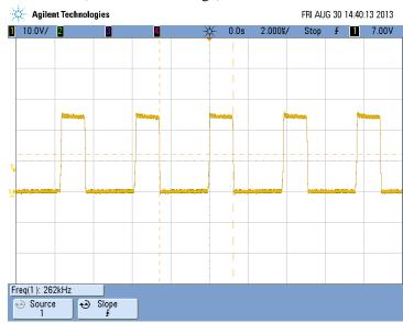
3. Test condition: The input voltage was set at 32V, and all four outputs were set at full load. Ch1 – Vd5 (+15V output diode voltage stress from cathode (-) to anode (+), 200V rating diode)
