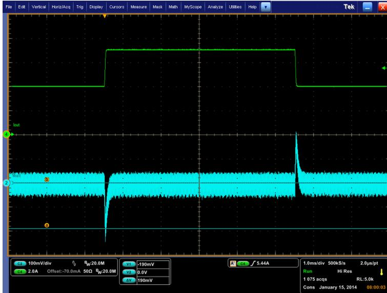
57V<sub>in</sub> @ 4A to 7A, 100mA/μs, Pulse f @ 100 Hz,
