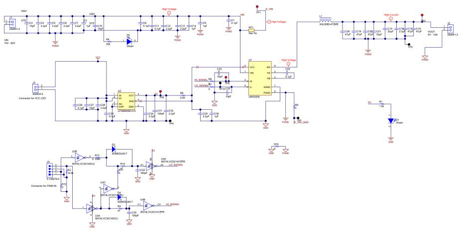
Figure 1. LMG5200EVM-01A Schematic
