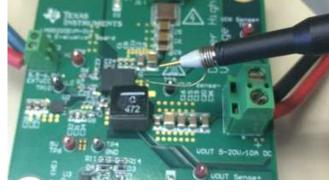
Figure 5. Measuring the SW Node
