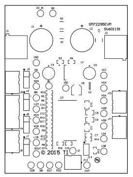
Figure 4. Top Assembly Layer
