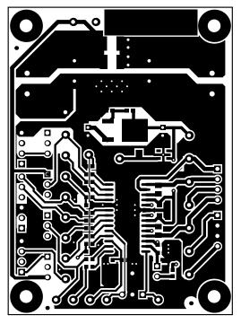
Figure 5. Top Routing Layer
