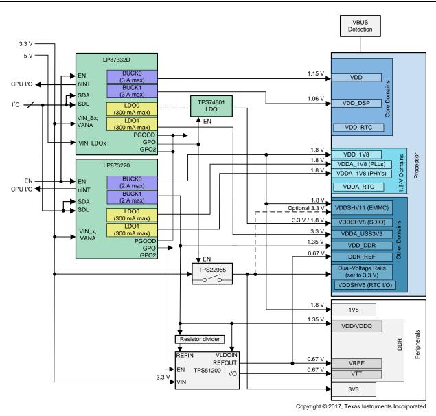
Figure 1. Processor Connection With LP87332D and LP873220
