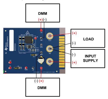
**Figure 1. EVM Board Connections**
