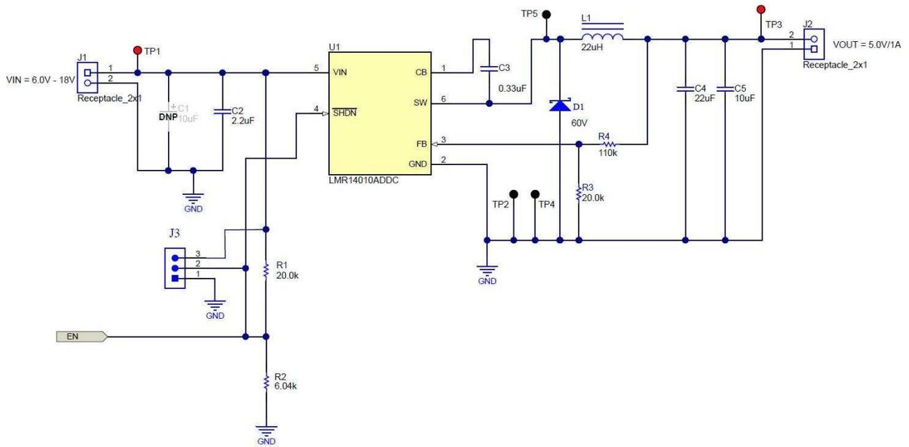
Figure 3. LMR14010AEVM Schematic
