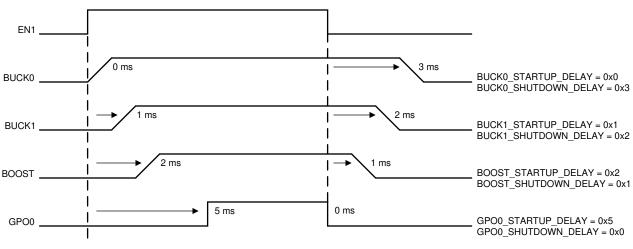
STARTUP\_DELAY\_SEL = 0x1 SHUTDOWN\_DELAY\_SEL = 0x1
